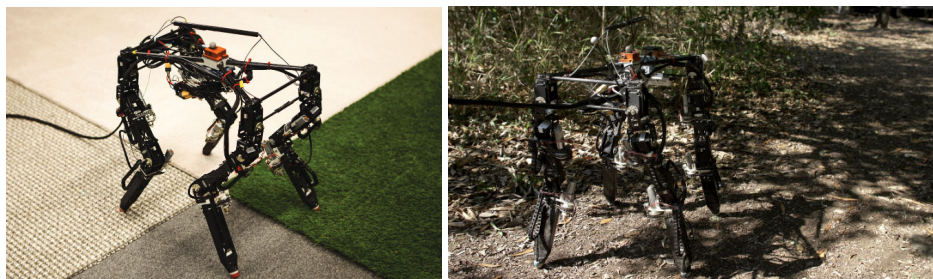
Figure 2: The robot on the four different walking surfaces is was tested on in our work on adapting to the operating environment in the lab [12] to the left. We showed that evolution was able to utilize both control and morphology to adapt to different environments. We also showed the results could generalize to new and unseen environments. The right shows the robot during testing of our online adaptation algorithm in outdoor unstructured terrains [13]. Here, the robot was able to exploit limited training in the lab to quickly and efficiently adapt its body to new and unseen environments.
