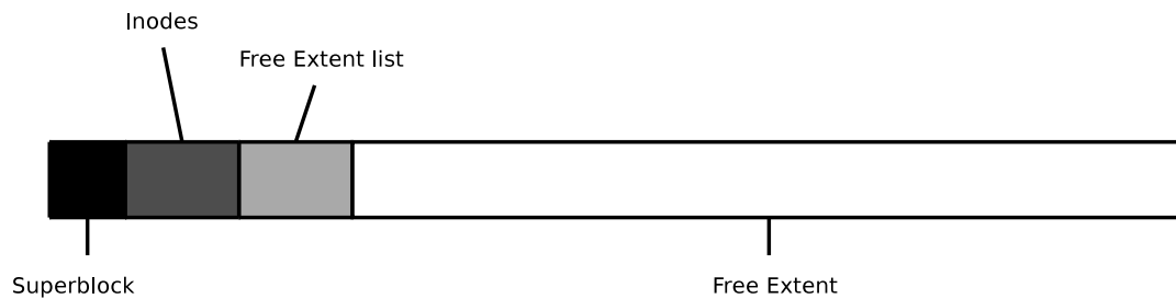
Figure 3.3: Disk layout on an empty file system
