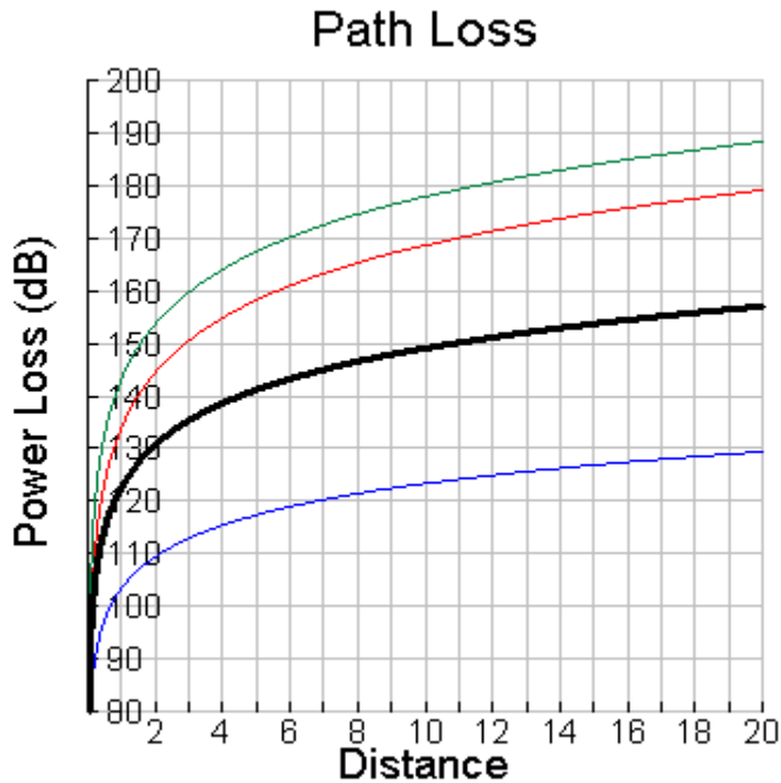
Fig. 47 The Path Loss model for WiMAX as a function of distance for NLOS measurements (thick line) from Eq. 22. FSL (bottom line), Cost 231 Hata Urban (topmost) and Cost 231 Hata Suburban (next topmost line)
