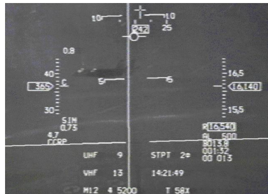
Figure 7.1: Illustration: The view from the cockpit of an F-16 fighter plane shows the HUD display. The lines in the centre shows the plane's direction and elevation, while the other elements display vital information such as airspeed and altitude. Newer versions of fighter pilot HUD's are mounted on the pilots' helmets instead of on the dashboard.
