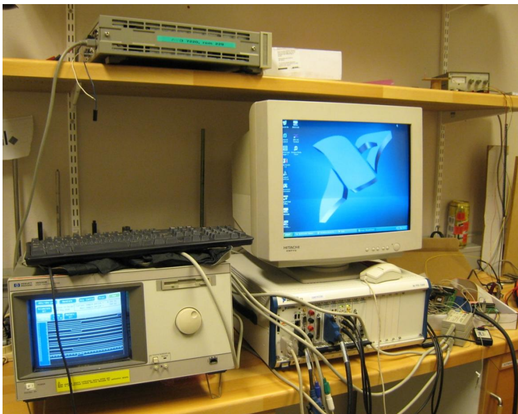
Figure 6-1 The test bench at the laboratory. On the left is the digital analyzer. The computer in the middle is the LabView computer. In the cardboard box to the right are the PCBs and the photo sensor circuit. On the shelf there are two power supplies. The photo is taken during testing of the digital signals.
