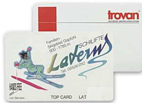
Figure 3.2: Skipass is a short-range passive RFID-tag. (Courtesy of Trovan Inc.)
