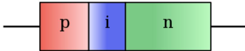
Figure 7.3: Photodiode with an un-doped intrinsic semiconductor material between the positive and negative doped layer.
