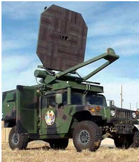
Figure 3.4: The ADS mounted on a Humvee (Courtesy of The Joint Non-Lethal weapons program.)
