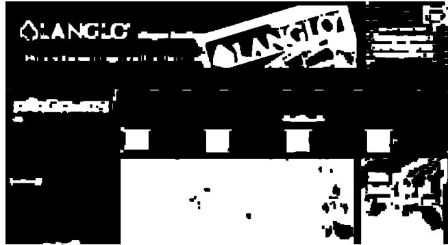
Figure 4.10: The segmented image before labeling the different picture regions. The white pixels belong to pictures.
