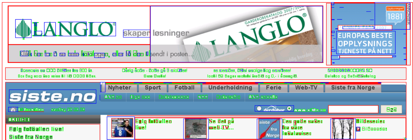
Figure 4.15: The different regions before merging. The blue regions are image regions, red are boxes and green are text regions.
