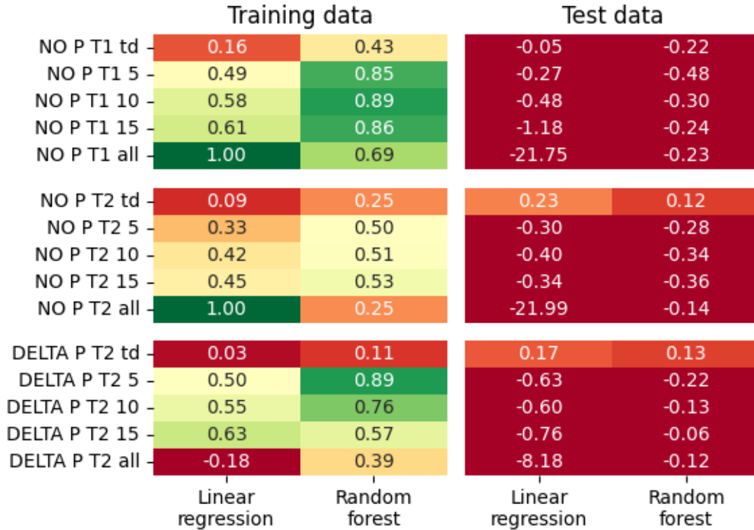
Figure 4-17: Coefficient of determination, R^2 , calculated from regression tasks done on various features spaces using multiple linear or random forest regression. The model was evaluated on the data used for training (left), and the hold-out testing data (right). The models were created using either only time and dose (td), or the best 5, 10, 15, or all, image features.
