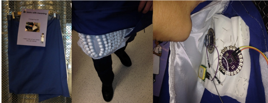
Fig. 2. The final concept for the skirt: simple wrap-around style with Velcro closure, balls for comfort and GPS sensor for motion tracking. Photos: Culén.
