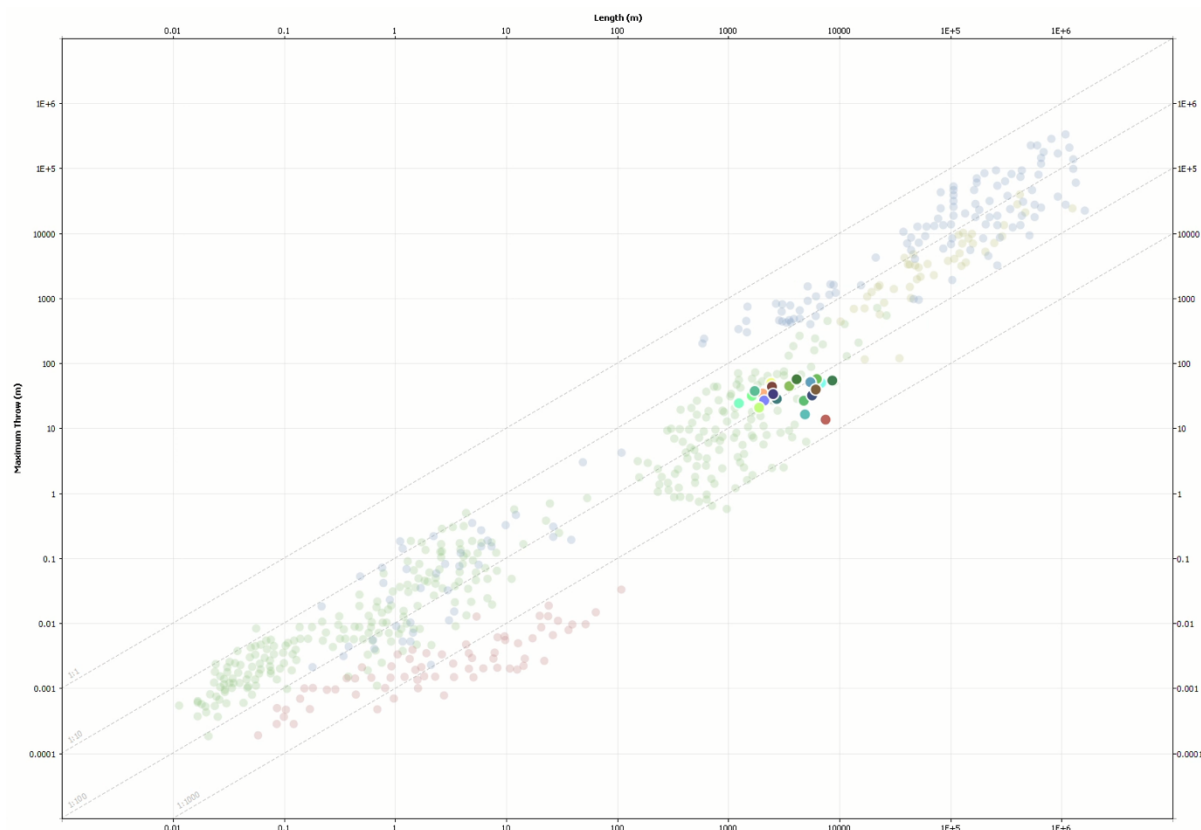
Figure 4.14. Maximum throw vs. length plot of 22 of the 36 faults within the study area. Global measurements of normal, thrust, strike-slip faults, and deformation bands are obtained from PETEX Move. Green plots are expected values for normal faults, yellow are thrust faults, blue a strike-slip faults, and red is deformation bands.
