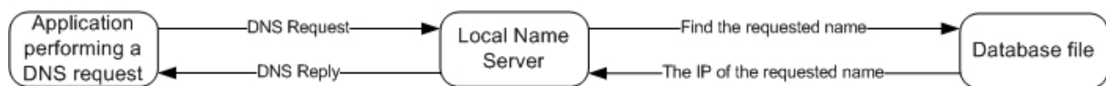
Figure 3.7: A local name resolution with a DNS server running on a local node.
