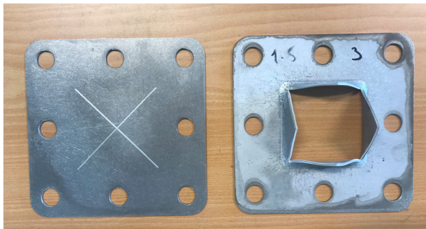
Fig. 2 Left-hand side: Picture of an aluminium membrane prior to test. Right-hand side: Aluminium membrane photographed after test
