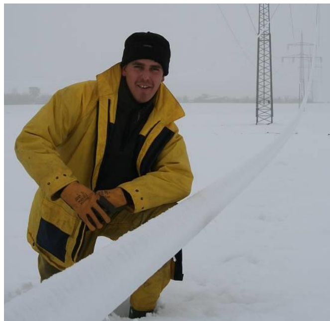
Figure 2.6: Wet snow ice on a cable in the Münsterland area, Germany, 2005. (Photo: Wichura and Kiessling (2009)).
