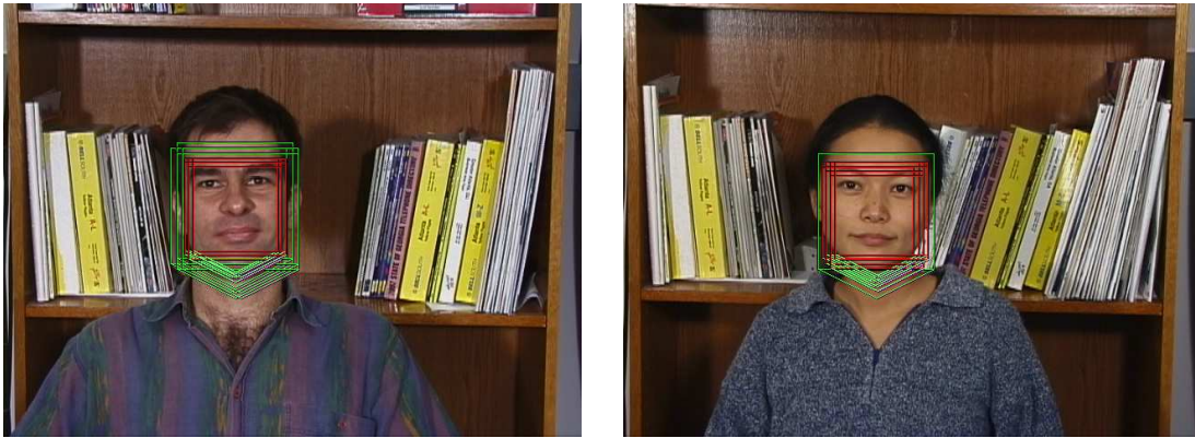
Figure 26: Output from face recognition. Green squares surround localized faces and red squares indicate a recognized individual
