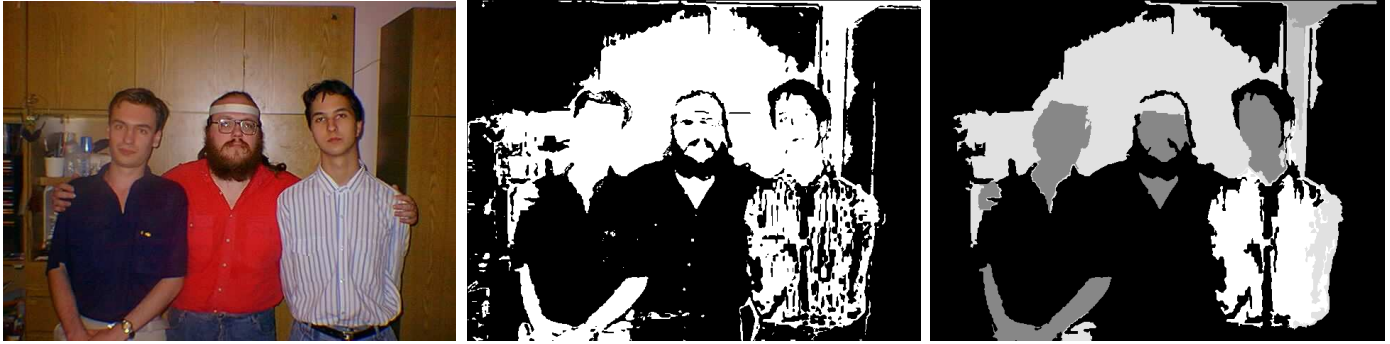
Figure 27: From the left: Input image, skin colour thresholded, result after histogram clustering and cleaning. While they are merged in one skin colour region after thresholding, all faces separated after clustering.
