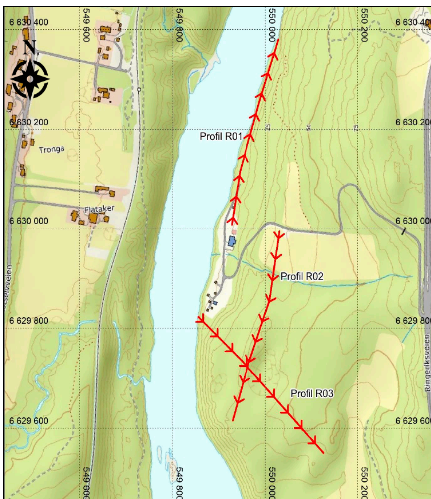
Figure 3.7. Location for geophysical methods (GPR and ERT).
