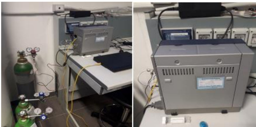
Figure 3-8 CP 4900 Gaschromatograph used to carry out laboratory analyses of soil gas samples, free gas and dissolved gas in the groundwater.
