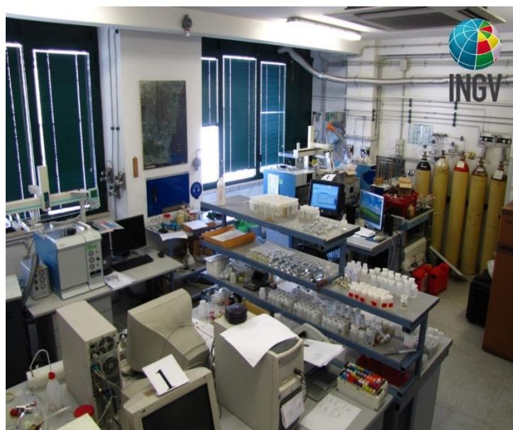
Figure 3-9 Image of stable isotope laboratory of INGV Palermo focussed on isotopic composition of hydrogen, carbon and oxygen ( \delta\text{D} , \delta^{13}\text{C} , \delta^{18}\text{O} ) on a variety of samples (soil, sediment, water, and atmospheric gas), by means GC-IRMS (Isotope Ratio Mass Spectrometry).
