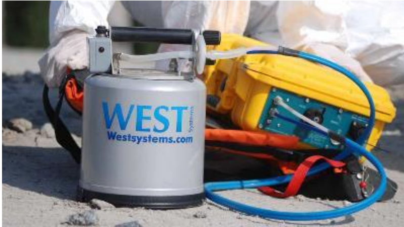
Figure 3-7 Photo of the West Systems™ portable fluxmeter with the logo printed on the accumulation chamber(WestSystems, 2020).
