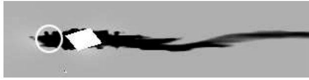
Figure 6.12: An artificial “tail” (marked with a circle) with small values in the velocity field in front of a moving object. The flowing obstacles flows from left to right. The tail must not be mistaken with the area with naturally small values in the cover of the obstacle.
