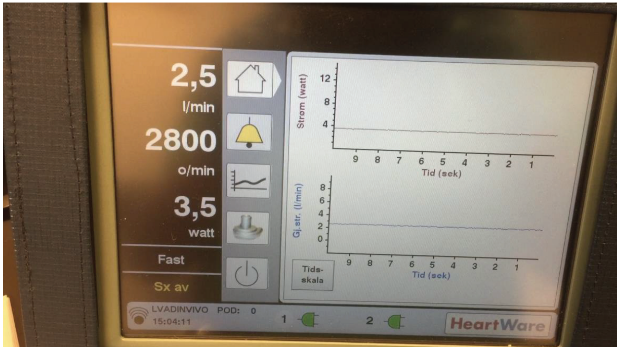
Figure 2. HeartWare HVAD monitor. The monitor presents continuous real time data. Pump power consumption (watt), estimated flow (l/min) and pump speed (RPM).
