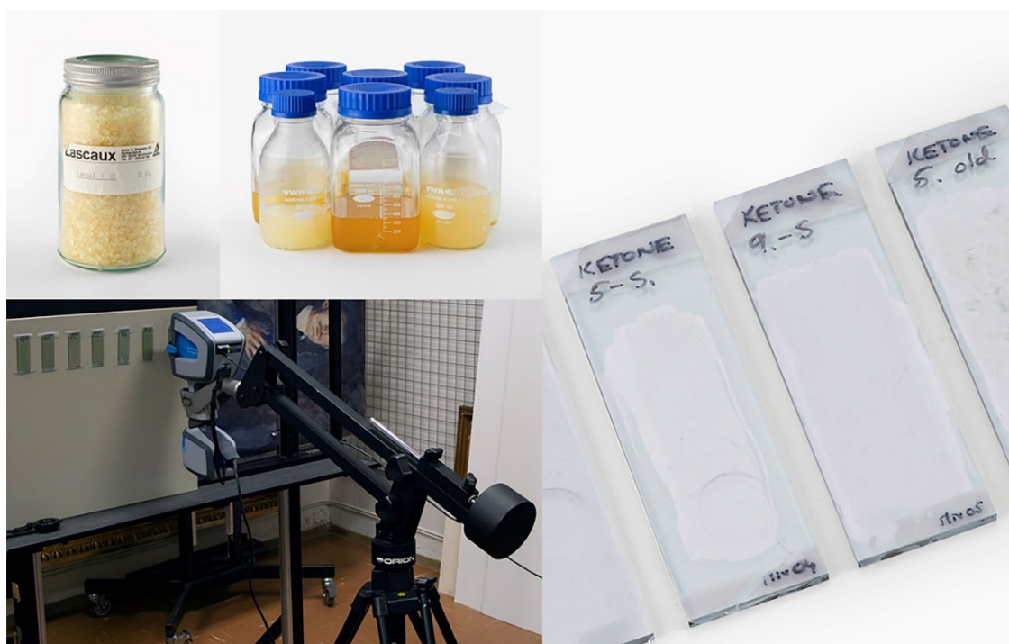
Figure 11. pFTIR (DRIFT) varnish library tests. Dry resin sample, recipe solutions, MirrIR low-e microscope slides and tripod set-up (2022/2018, Nasjonalmuseet/Ford)
