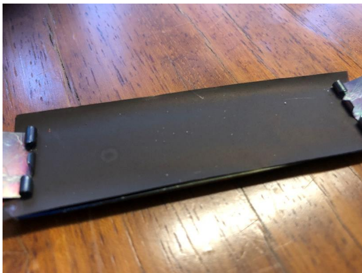
Figure 14: Si electrode strip attached to a Si-wafer using paper clips.
