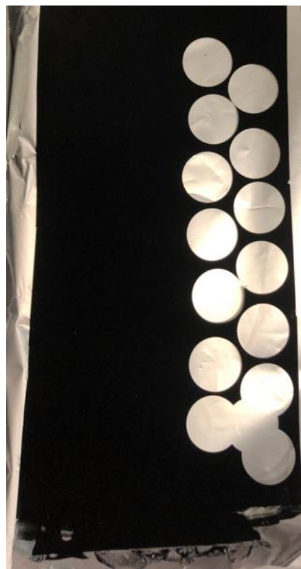
Figure 10: AC electrode tape with holes where electrodes have been punched out.
