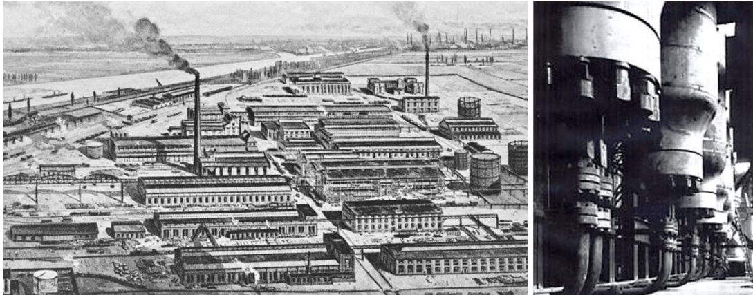
Figure 3. Left: The first Haber-Bosch ammonia production facility located in Oppau, Germany. The picture is a reproduction of a painting by Otto Bollhagen from 1914, reused with permission from BASF [8]. Right: A high pressure reactor for ammonia synthesis from the plant at Billingham, reused with permission from Johnson Matthey Plc [2].
