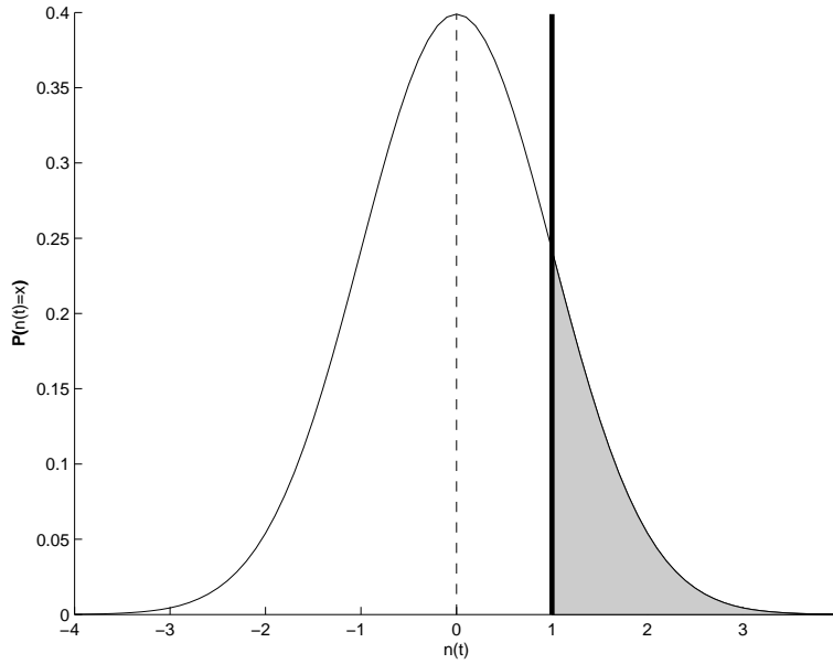
Figure 2.6: Shows the PDF of a noisy input in the absence of a signal with \sigma_n = 1 and \hat{\theta}_t = 1 . The colored area represents the P_{fa}
