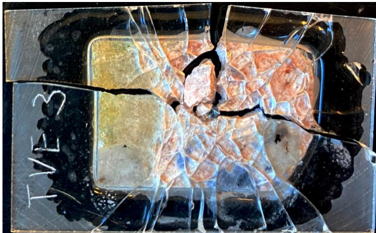
Figure 4: An example of one of the fragmented thin sections from thin section preparation.
