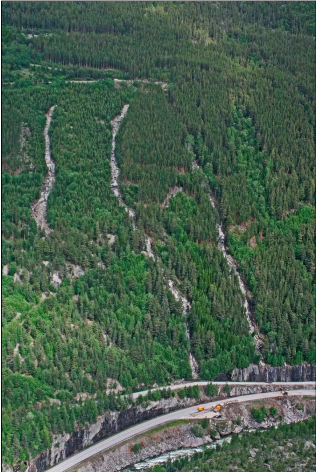
Figure 1.5 - Runout tracks from the three landslides in Høvringslia, June 10 th , 2011. Photo from Walberg & Devoli (2014).
