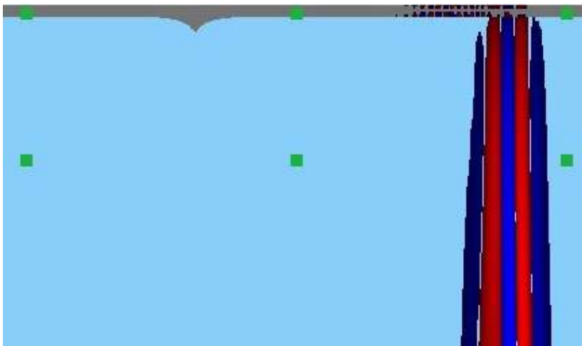
Figure 62. The wave field at 0.89 s for the ice model with the shallower ice ridge at x = 996 m. The wave in the ice layer appears weaker than for the corresponding model with a deeper ice ridge at the same location in Figure 61. Also, the wave seems to propagate more in the ice and not in the ice-water interface.
