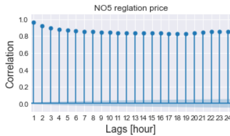
Figure 4.13: Autocorrelation of the regulation price for bidding zone NO5 over 2016-2021 data
