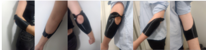
Figure 9: Sockets being worn by the two test subjects. One socket had to be cut at the bottom to allow for donning and doffing comfortably.
