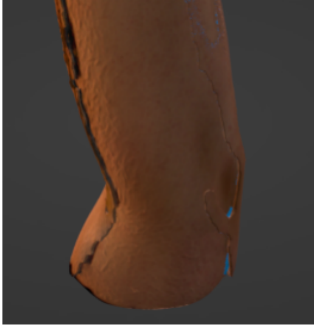
Figure 5: Surface corruption in the interest area resulting from the loss and subsequent recovery of tracking.
