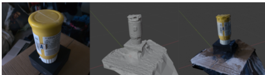
Figure 4: Our first attempt at photogrammetry. Left to right: one of the photographs used, untextured mesh, textured mesh.
