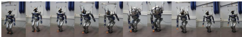
(b) HRP-2 picks up the ball between its feet. "stepping away" is a direct consequence of the action "pick up the ball". Indeed, there is no dedicated module in charge of stepping away but it is part of the module "pick up the ball".
