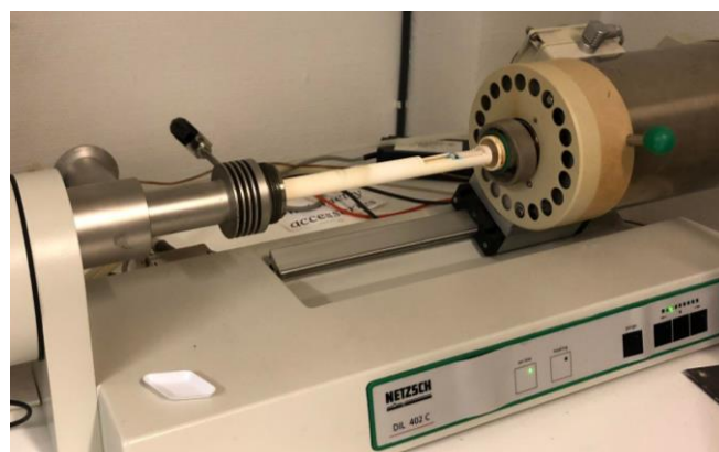
Fig. 11: NETZSCH DIL 402C Dilatometer
