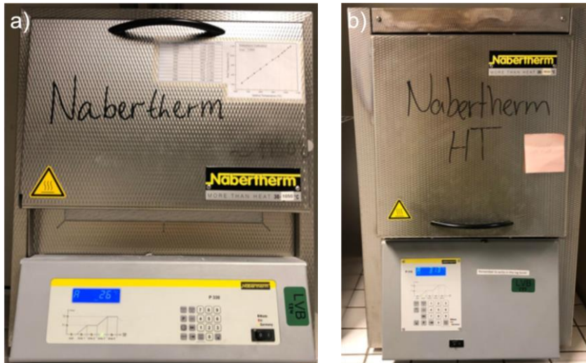
Fig. 10: Picture of muffle furnaces, a) Nabertherm LVB524 b) Nabertherm HT LVB533
