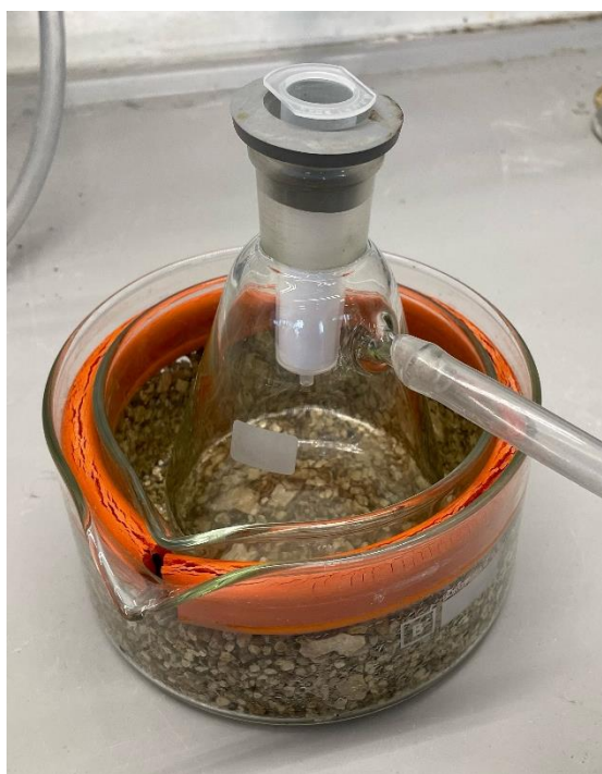
Picture 2.1: Purification setup of a short plug with suction used for purification in bromination reaction of diazo compounds.
