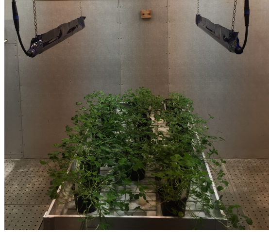
Figure 5: Experimental set-up at the beginning of Experiment 2. Twilight was mimicked by two LED tubes covered with blue filters. As the Trifolium repens grew larger, the pots were distributed on two tables.
