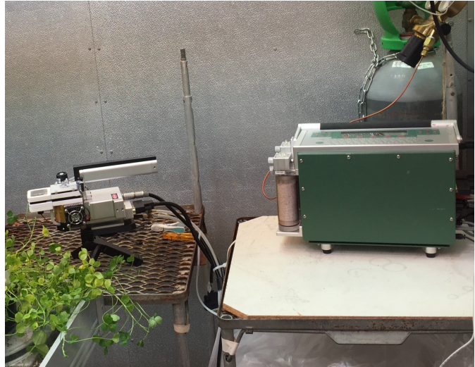
Figure 6: Set-up for the diurnal measurements of Trifolium repens , using an LI6400 portable photosynthesis system. A 40 L gas cylinder was used as CO 2 source, and air from outside the phytotron room was conveyed through a plastic tube to the air intake of the instrument. During the measurements, the plant pot stood in a plastic tray with water on the watering table, while one leaf was held in the LI6400 sensor head (with a standard 2x3 cm leaf chamber) on an adjacent table.
