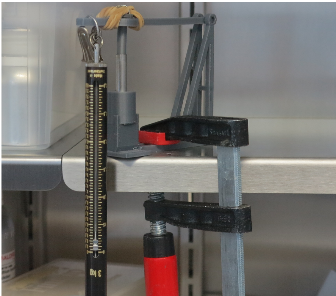
Figure 3.7: Powderpress setup used for ARC sample preparation
