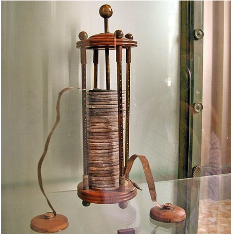
Figure 1.1: Alessandro Volta's electric battery (Tempio Voltiano in Como, Italy) by GuidoB. CC Attribution Alike 3.0 Unported license
