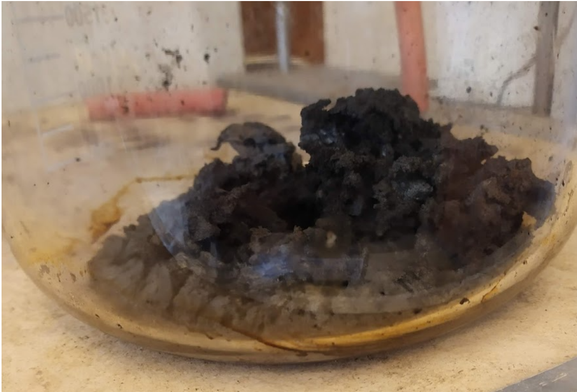
Figure 4.1: Sol-Gel combustion synthesis of the Al_{0.2} -Mn sample
