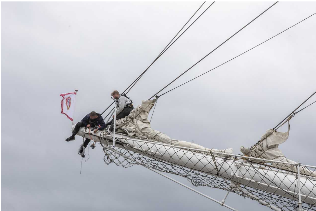
Figure 3.1: Mounting of the ultrasonic altimeter probe 1 under the bowsprit tip on the 16.06.2021 in Bergen/ Norway (Picture by Marita Aarekol).
