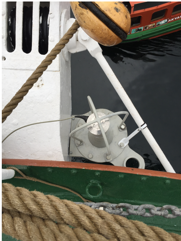
Figure 9: The radar probe mounted on the starboard side of the bow, with the empty slot for ultrasonic probe 2.
