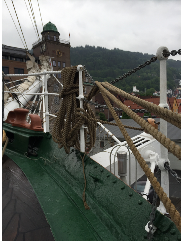
Figure 8: The radar probe mounted on the starboard side of the bow.
