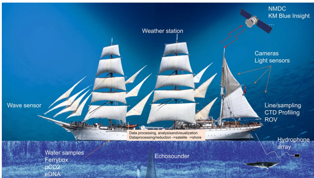
Figure 3.4: Research instruments and system installed on board the Statsraad Lehmkuhl for the One Ocean Expedition (2021-2023) (One-Ocean-Expedition-website, 2022).
