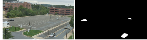
Figure 1: Segmentation result of cars, which is suited to be used as an SDR. Original frame taken from VIRAT [16].
