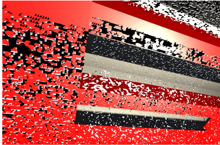
Figure 4.12: Graphical artifacts caused by compute buffer overflow within a single update when using too conservative memory-saving settings. Left upper corner: area of the corrupted triangles. Right lower corner: stretched corrupted triangle.
