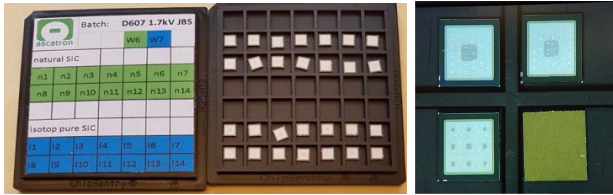
Fig. 3. Left: Box with bare die diodes, 14 natural SiC, and 14 monoisotopic SiC. Right: Close up of four diodes, bottom right shows cathode/backside, the three others show anode/front side.
