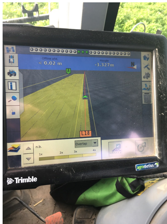
Image 6. Roy, Simon O. 2021. The interface of the RTK navigation system in Daan's tractor.
