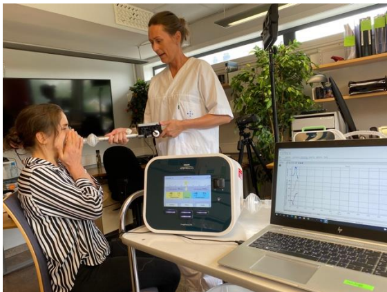
Figure 2. MI-E intervention. Research physiotherapist testing one of the subjects. The research physiotherapist is holding the pneumotachograph with the tube and filters and the subject gives support to the mask to avoid air leakage. Consent for publishing this photograph was given from the participant.
