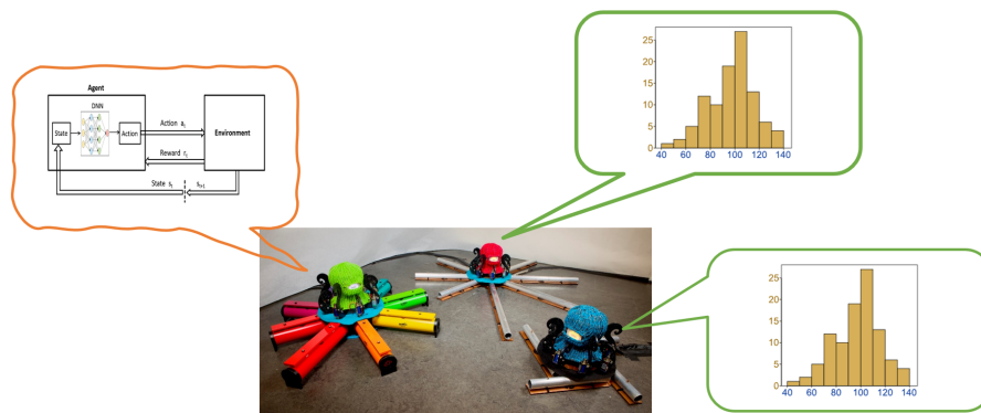
Fig. 1. Dr. Squiggles robots setting. We have used two Dr. Squiggles robots with a histogram-based rhythm generating algorithm in the environment. The agent is the third robot and uses a DRL algorithm to learn the rhythmic patterns from the environment.
