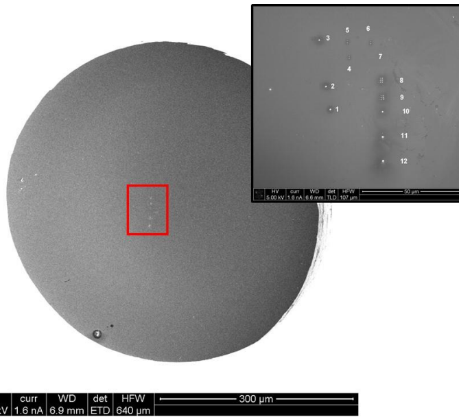
Example for 6a of the overview of deposits in the hole of the vapour guide.
