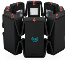
Figure 1.1: Myo armbands have been used in several of the projects presented in this dissertation. It is a (now discontinued) commercial sensor interface containing eight electromyogram (EMG) electrodes, an inertial measurement unit (IMU), and wireless communication over Bluetooth.
