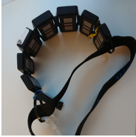
Figure 3.3: The modified Myo armband to fit around the calf of the dancer.
