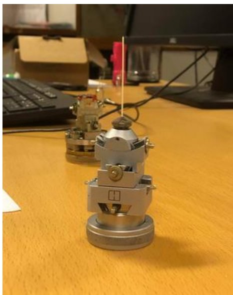
Figure 4-2: Illustration of how a capillary tube with sample is mounted on a station for capillary XRD.
