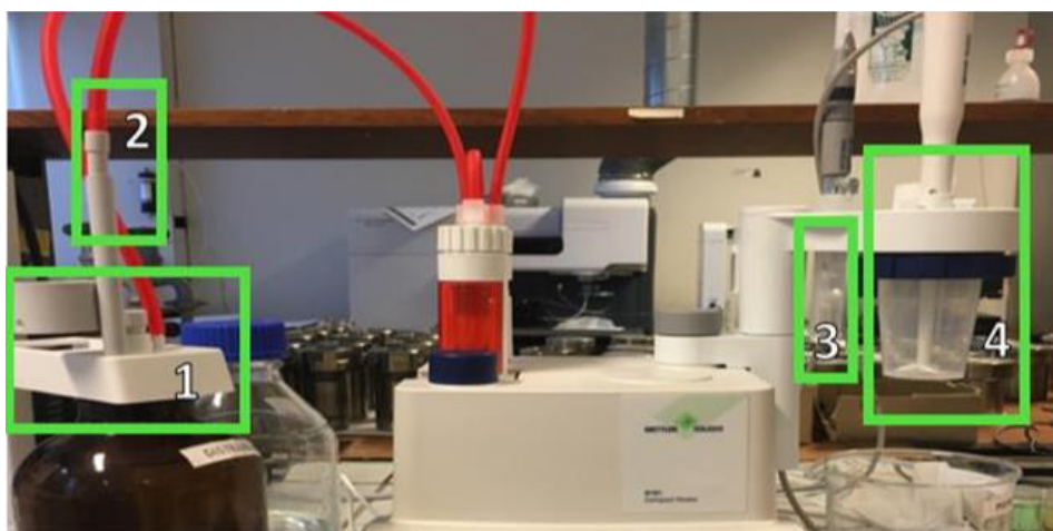
Figure 4-9: Illustration of set up for the potentiometer, where 1 is burette feed, 2 is burette tip, 3 is pH – electrode in stand with 3 M KCl – solution and 4 is the titration stand. Adapted from (12).
