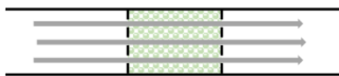
Figure 3-12: Scheme of a plug flow reactor, where the flow is indicated as 3 grey lines.
