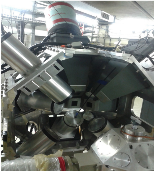
Fig. 5. The AFRODITE array consisting of HPGe clover detectors with BGO shields, large volume 3" by 8" LaBr 3 :Ce detectors and medium sized 2" by 2" LaBr 3 :Ce detectors.
