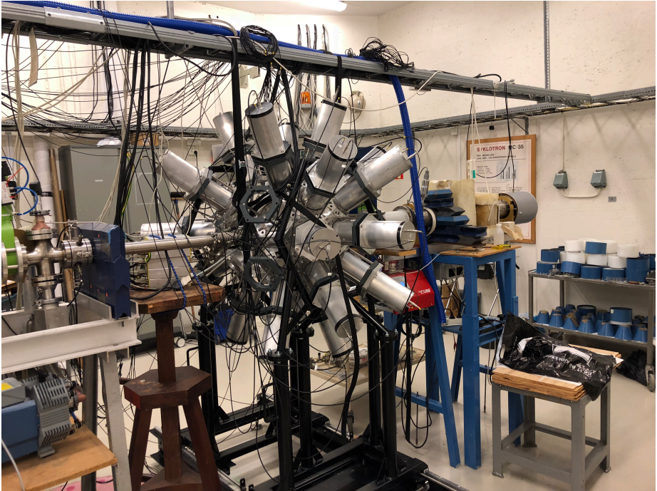
Figure 3.1: The OSCAR \gamma -detector array consisting of 30 large-volume \text{LaBr}_3\text{:Ce} detectors.
