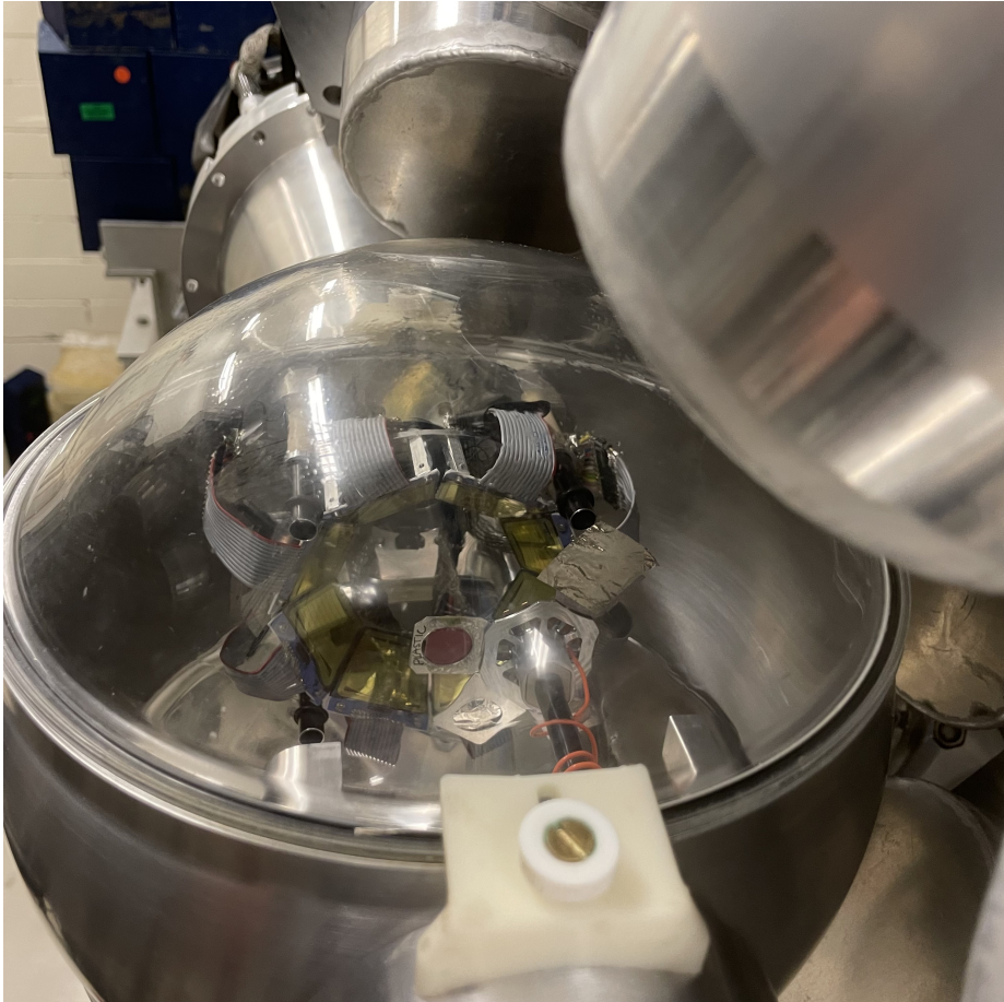
Figure 3.2: New target chamber made for the OSCAR array. A variety of targets are mounted on the target wheel in front of the SiRi particle telescope.
