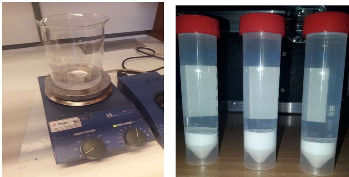
Figure 3.1. Left; The beaker containing BaCl_2 and deionized water solution placed in a magnetic stirrer. Right; the centrifuge tubes with the precipitate of BaSO_4 settled at bottom and clear solution of NH_4Cl at the top.
