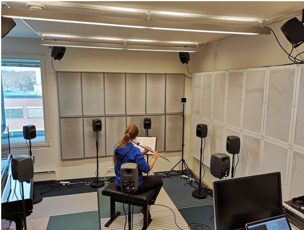
Figure 4.23: View of the virtual reality lab at the Norwegian Academy of Music. One performer is seated surrounded by 12 loudspeakers but without the virtual reality headset.
