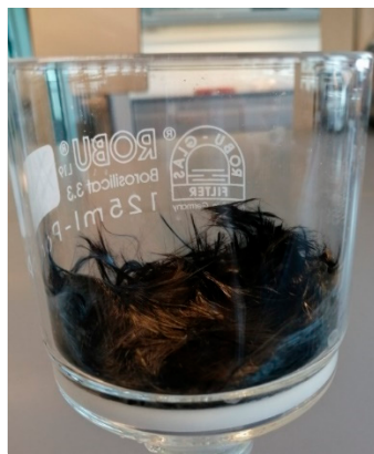
Figure 4. Remaining carbon fibers in the filter after the etching process.
