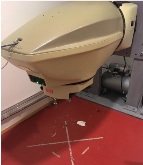
Figur 3.5: Radiumhospitalets gammakilde Gammabeam X200, MSD Nordion (serienr. 006) .
