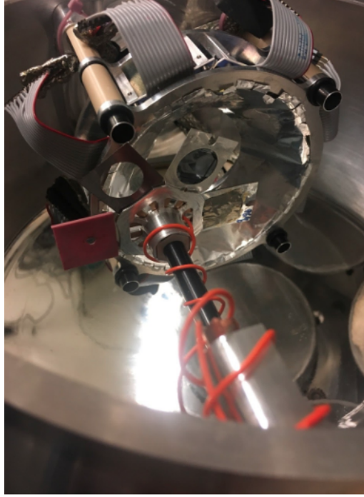
Figure 3.3: A picture of the SiRi particle telescope set up for the ^{28}\text{Si}(p, p') experiment.
