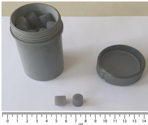
Figure 17: the Teflon cup and agate pellets used during the wet milling of the samples. The sample and ethanol are poured on top of the pellets and the cup is firmly closed before inserting it in the micronizing mill.
