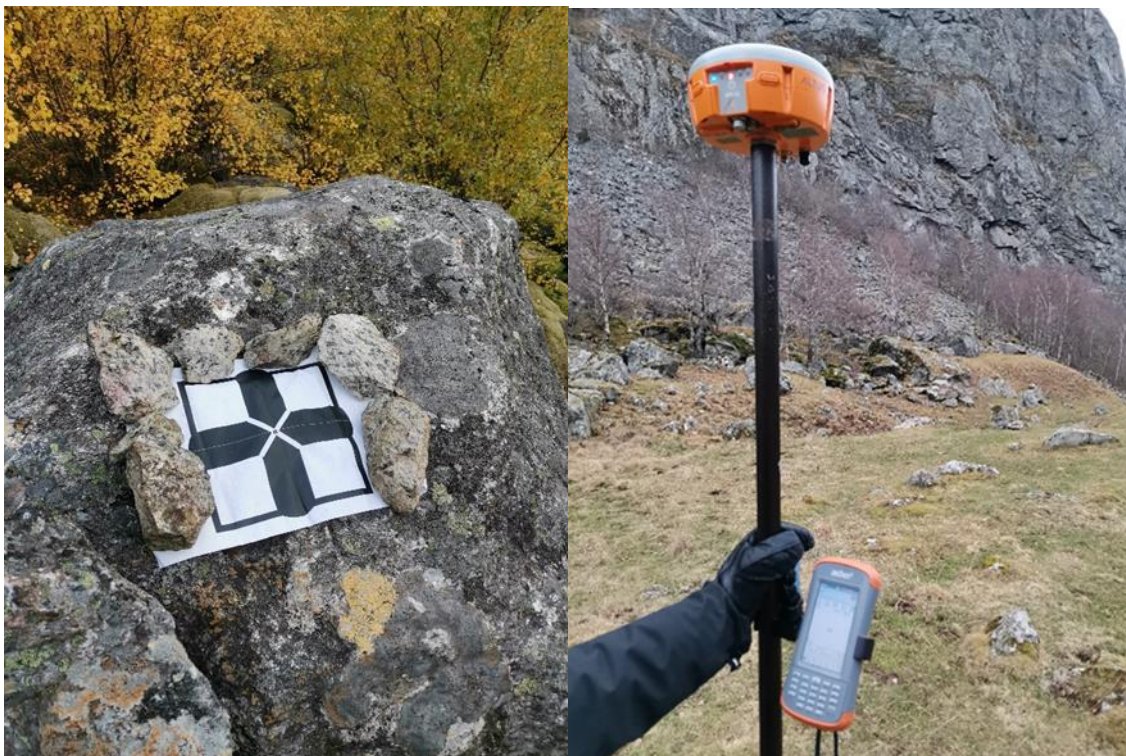
Figure 4.1 Left) a ground control point (GCP) on a boulder, marked with a cross. Right) the GNSS device (Altus APS-3G) used to record positions of the GCPs. The GNSS device is mounted on a pole, with the field computer attached to it.
