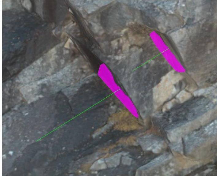
Figure 4.5 Illustration of output from a discontinuity spacing analysis in Maptek PointStudio. The pink planes represent discontinuity surfaces and have been reoriented according to the mean orientation of the discontinuity set. The green lines represent the distance between adjacent planes, normal to the mean orientation of the discontinuity set.
