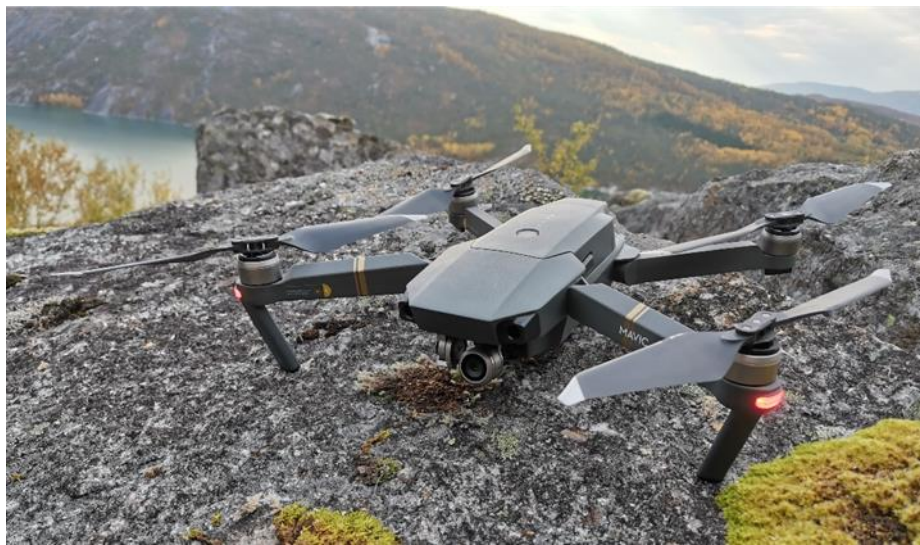
Figure 4.2 DJI Mavic Pro drone was used to perform the photogrammetric surveys. The drone was provided by the University of Oslo.
